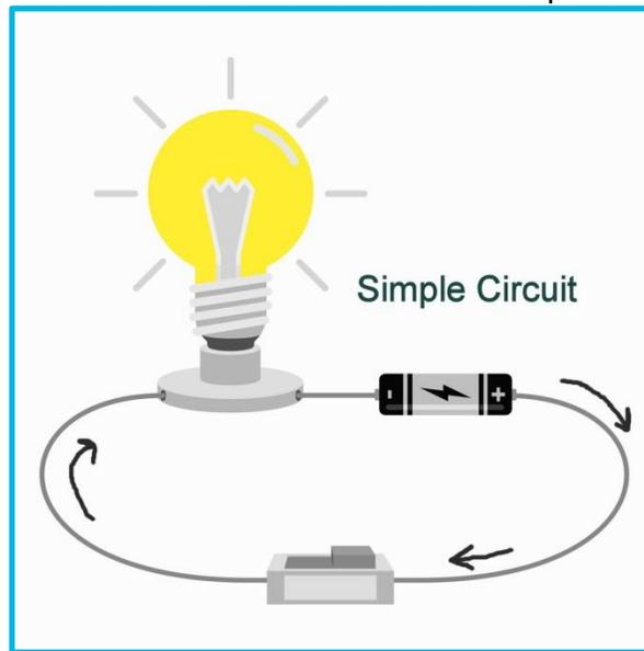
◆ **Schematic Diagram of a Simple Circuit**
